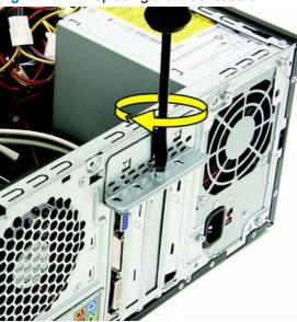
Figure 2-24 Replacing the bracket screw
